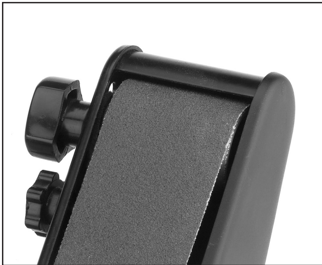
Figure 8. Sanding belt centered between belt cover edges at the upper roller.
